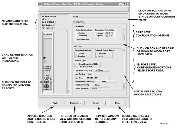
Figure 747-1. E1 Multi 1 Card Configuration Window
